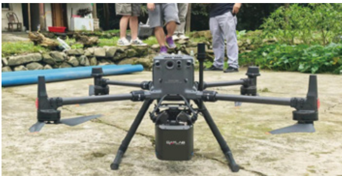
Figure2 SatLab Apus-MX mounted on the DJI M350
