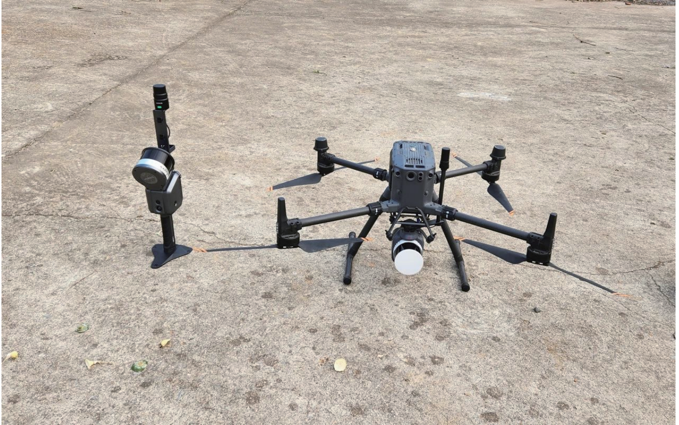
Figure 4 The LixelX1 SLAM scanner and APUS integrated with DJI M350RTK
