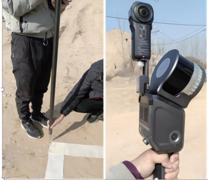
At the same time, operators can also view the acquisition path, relative position, laser point cloud effect, control points list, as well as the situation of incorrect or missed scanning in real-time through Lixel GO APP. The onsite scanning takes 15 minutes.
