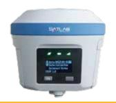
Signal Tracking GPS: L1, L2, L5
