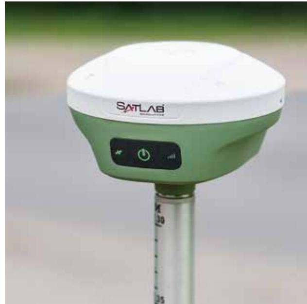
**Step 2.** Use Satsurv to configure Freyja as a base station under data collector internet mode. Therefore, Freyja is now officially a base station and will send correction data to the handheld terminal via Bluetooth.
