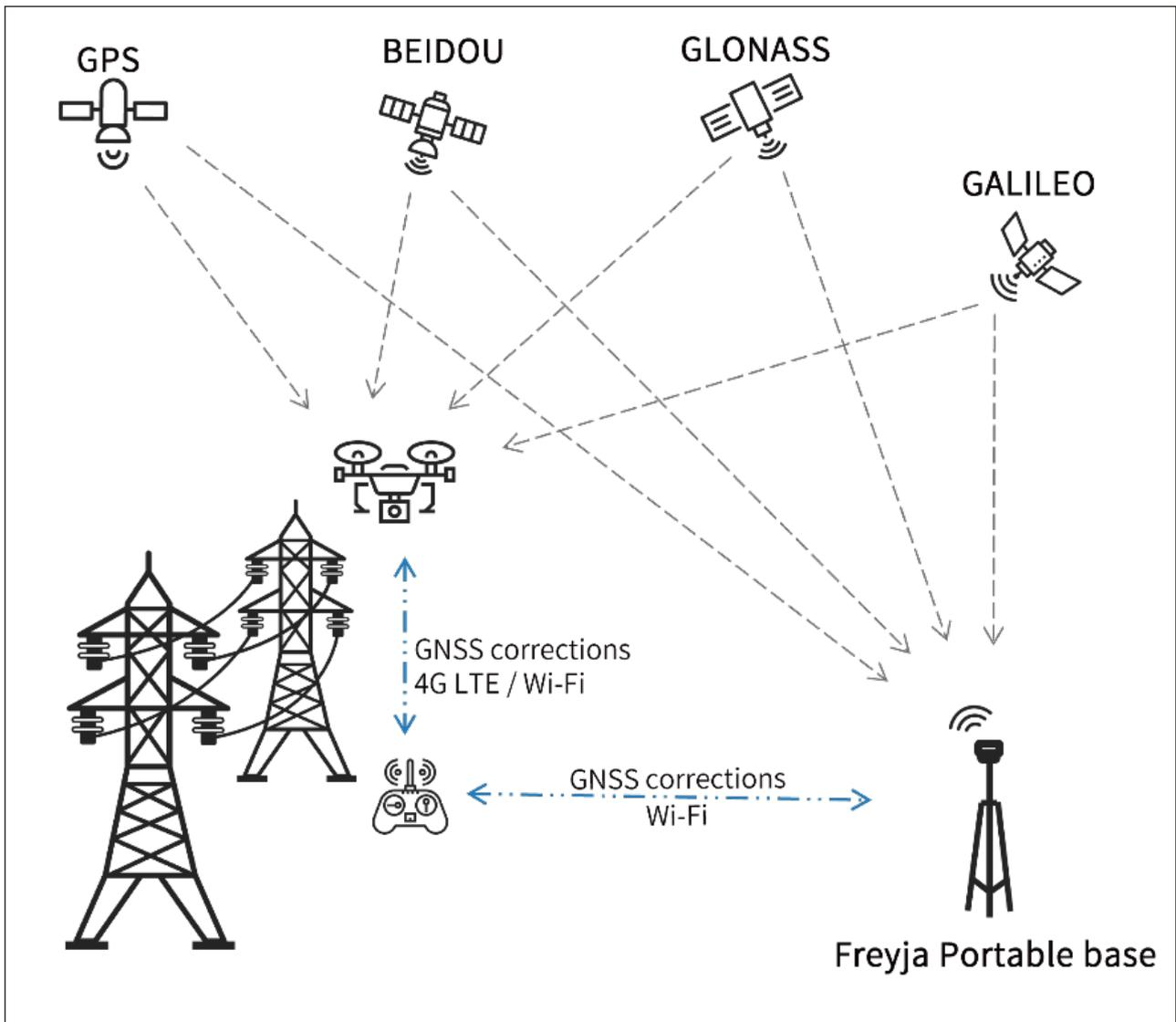
High-precision positioning and navigation is critical part of UAV drones regardless of the applications. Different from traditional drone surveying, the emergence of RTK technology such as Freyja GNSS receiver improves the work efficiency by offering real-time, highly-accurate position solutions for drone surveying, and ensuring a safer and more stable flight.
